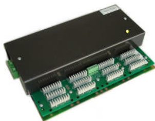
Area controller with 32 hard-wire & 100 wireless inputs
