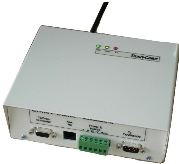
Master control (system polling) unit including Paging & Annunciator encoder and 100 channel wireless receiver
